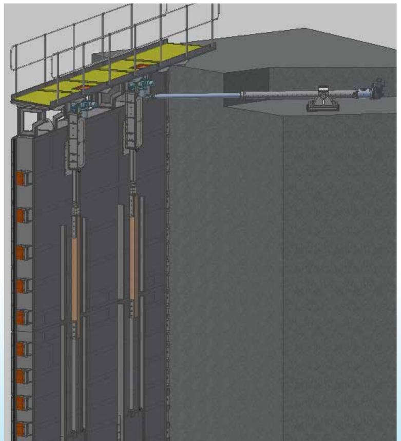
Caledonian Canal mitre gate with KGAL designed electric main gate actuator and sluice gate actuators
