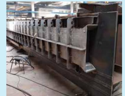
The trash rack 'flounder' and wheeled gate embedded track in fabrication in Riga
